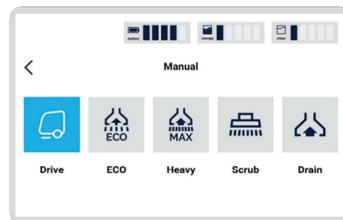
Here are 5 states in Manual Cleaning: Drive, ECO, eavy, Scrub, Drain
