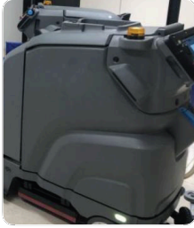
Front monocular scanning (Robot needs to be facing the QR code)
